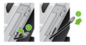
Using a credit card, gently pry up one edge of the hardware integration pocket insert, and then remove the insert.
